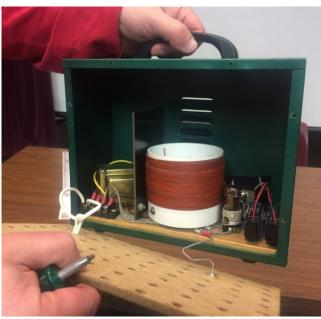
1 Tube Am Radio Receiver by Robin VE4IO
