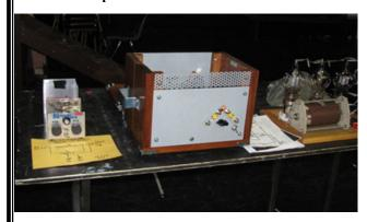
Another neatly constructed and well-labeled project was produced by Rolf VE4VZ. His "CL – LC switched tuner" features a roller inductor and tunable capacitor which can tune from 160 to 6 metres.
