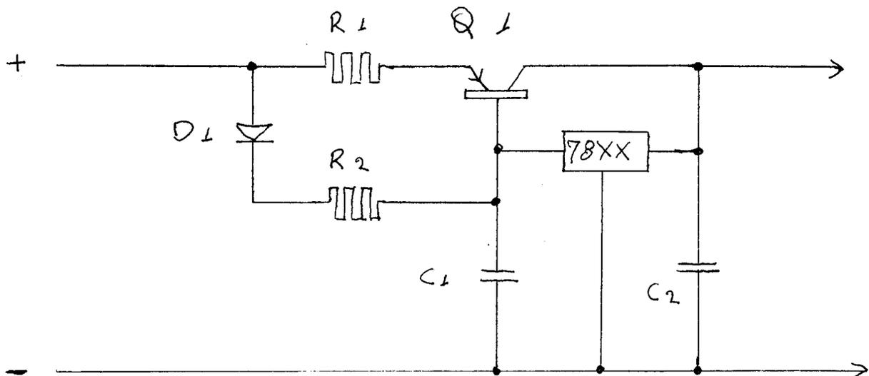
This is a circuit I have been using to increase current from a regulating chip like the 78xx series.
